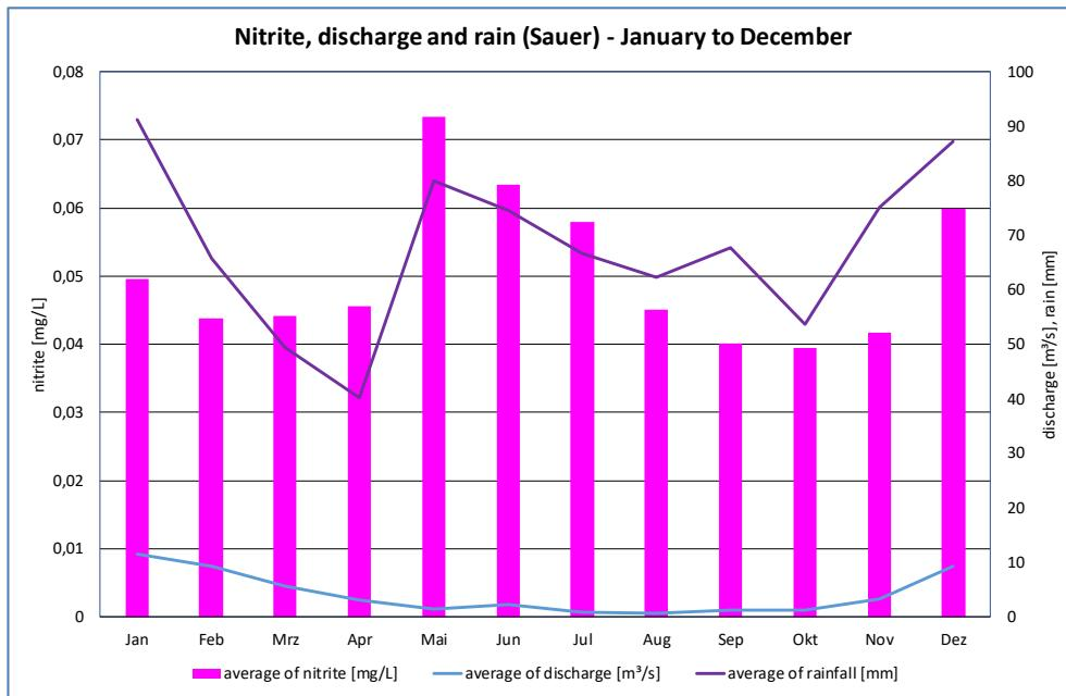
figure 18: Nitrite concentration compared with discharge and rain –January to December in the river Sauer
