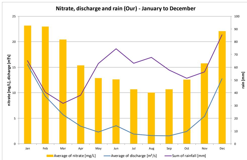
figure 5: Nitrate concentration compared with discharge and rain –January to December
