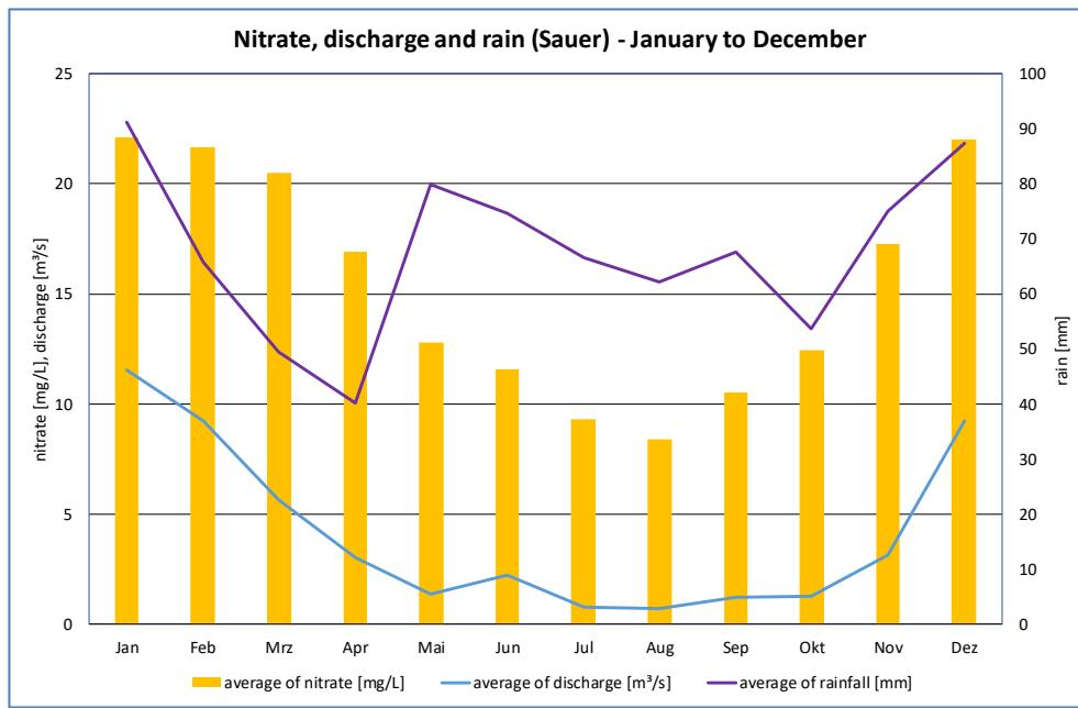
figure 14: Nitrate concentration compared with discharge and rain –January to December in the river Sauer
